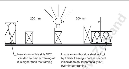
On the left hand side the top of the ceiling joist is lower than the top of the insulation and does not fully shield the insulation. The full clearance needs to be maintained. On the right hand side a smaller clearance is acceptable as the insulation is fully and permanently shielded by timber framing (provided the insulation material cannot potentially loft over the top of the ceiling joist – where this is not guaranteed the full 200 mm clearance shall be maintained).
