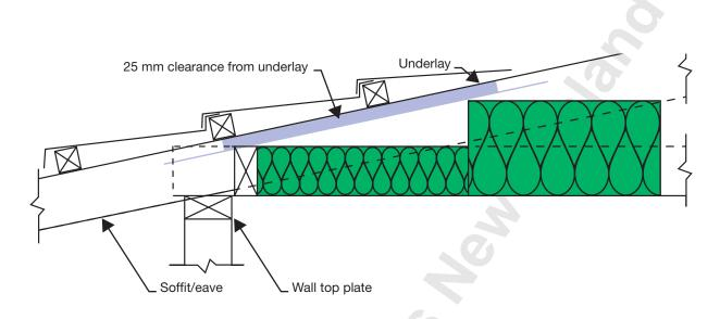
Figure 22 – Roof detail for a low-pitch roof
