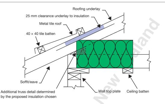
Figure 26 - Metal tile roof
