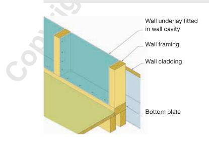
Figure 18 – Retrofitting wall underlay
