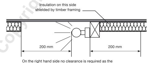
insulation is fully and permanently shielded by timber framing.
