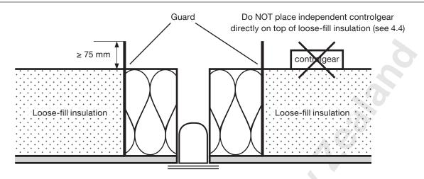
Figure 4 – Installing new loose-fill ceiling insulation around recessed luminaires of the type CA 80, CA 90, and CA 135 where the luminaire manufacturer's instructions are not known
