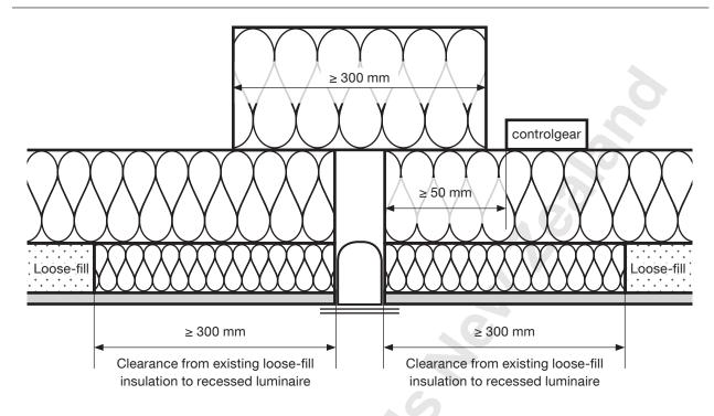
Figure 6 - Installing ceiling insulation around recessed luminaires of the type IC, IC-F, and IC-4 where the luminaire manufacturer's instructions are not known (ceilings with existing loose-fill insulation)
