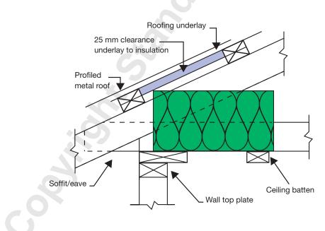
Figure 25 – Profiled metal roof
